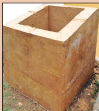
Figure 3: Proto type in-situ cast Mud-Concrete load-bearing wall models made for laboratory testing
