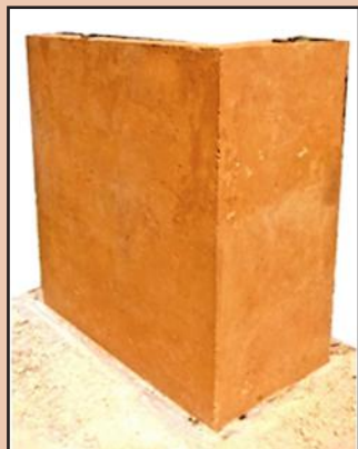
Figure 1: In-situ cast Mud-Concrete load-bearing wall segment
